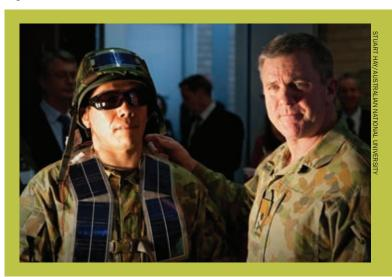
These lightweight solar panels, developed in Australia, stick to a Soldier's uniform and can be used to generate power in the field.
